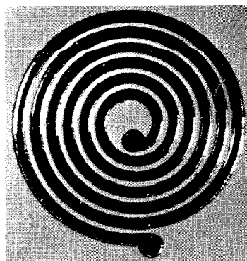
FIG. 2 - Photograph of 25 nh inductor (0.060" diameter)
